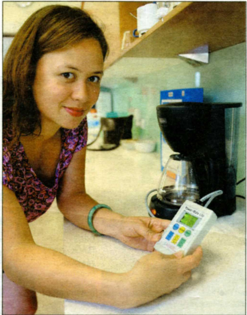
Sonya Tirtajaya with the Power Mate Lite, a device for measuring the energy consumption of household electrical appliances
